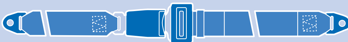
Standard static lap strap with flat anchor plates and fixed length webbing buckle.
